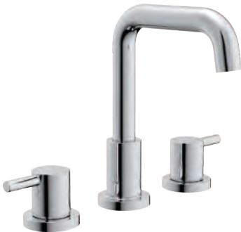
T80246 8" widespread lavatory faucet Zinc handle Brass spout Ceramic disc cartridge Metal waterway
