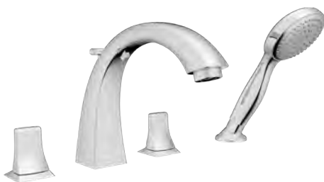
T20274 4-hole roman tub filler faucet Zinc handle Brass construction 16 points broach brass ceramic dis cartridge Single setting ABS hand shower
