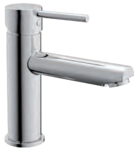
T80233 Single control lavatory faucet Zinc handle Brass construction Ceramic disc cartridge (Φ35)
