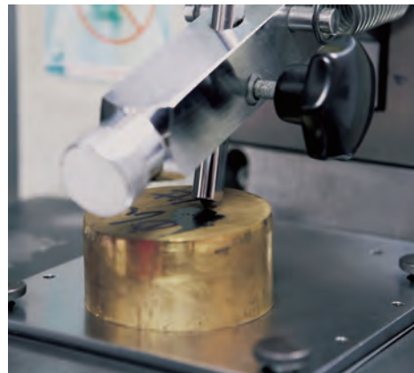
Spectrometer Analysis for metal composition
