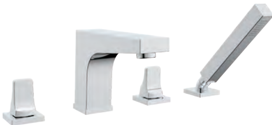
T80574-1 4-hole roman tub filler faucet Zinc handle Brass construction 16 points broach brass ceramic disc cartridge Single setting ABS hand shower
